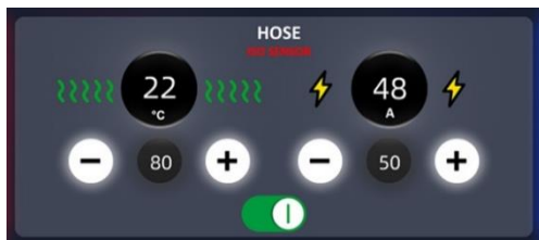
Individual hose heater (1 transformer / 1 probe)
